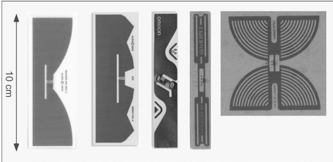
Figure 7.24: Commercial Broadband Structures, Approximately to Scale. (From left: Alien Technology (2), Omron, Rafsec (2)).
